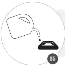
**WAIT FOR THE ELEMENT TO DRY AND MOISTEN IT WITH CLEAN ENGINE OIL. THEN IT MUST BE SQUEEZED TO REMOVE THE EXCESS OIL;**
