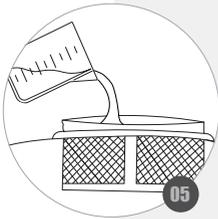
**INSERT INTO THE CHEMICAL TANK THE ALREADY DILUTED PRODUCT (BY PASSING IT THROUGH THE FILTER) AND IN THE QUANTITY NECESSARY TO CARRY OUT THE WORK;**
