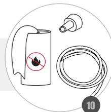
**USING A WET CLOTH WITH NON-FLAMMABLE SOLVENT, CLEAN THE METAL PARTS OF THE ENGINE;**
