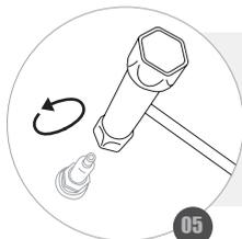
**REMOVE THE SPARK PLUG, PUT ABOUT 5ml OF CLEAN ENGINE OIL INTO THE CYLINDER;**
