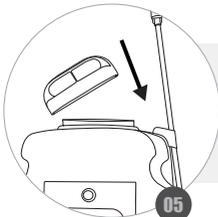
**REPLACE CHEMICAL TANK CAP BY TAPPING FIRMLY;**
