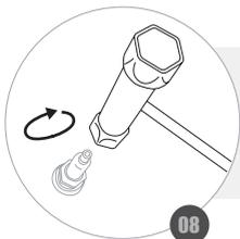
**AFTER SETTING THE SPARK PLUG, TIGHTEN WITH A WRENCH ABOUT 1/8 TO 1/4 TURN;**
