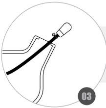
**WITH THE AID OF A HOOK, REMOVE THE FUEL FILTER OUT OF THE TANK;**
